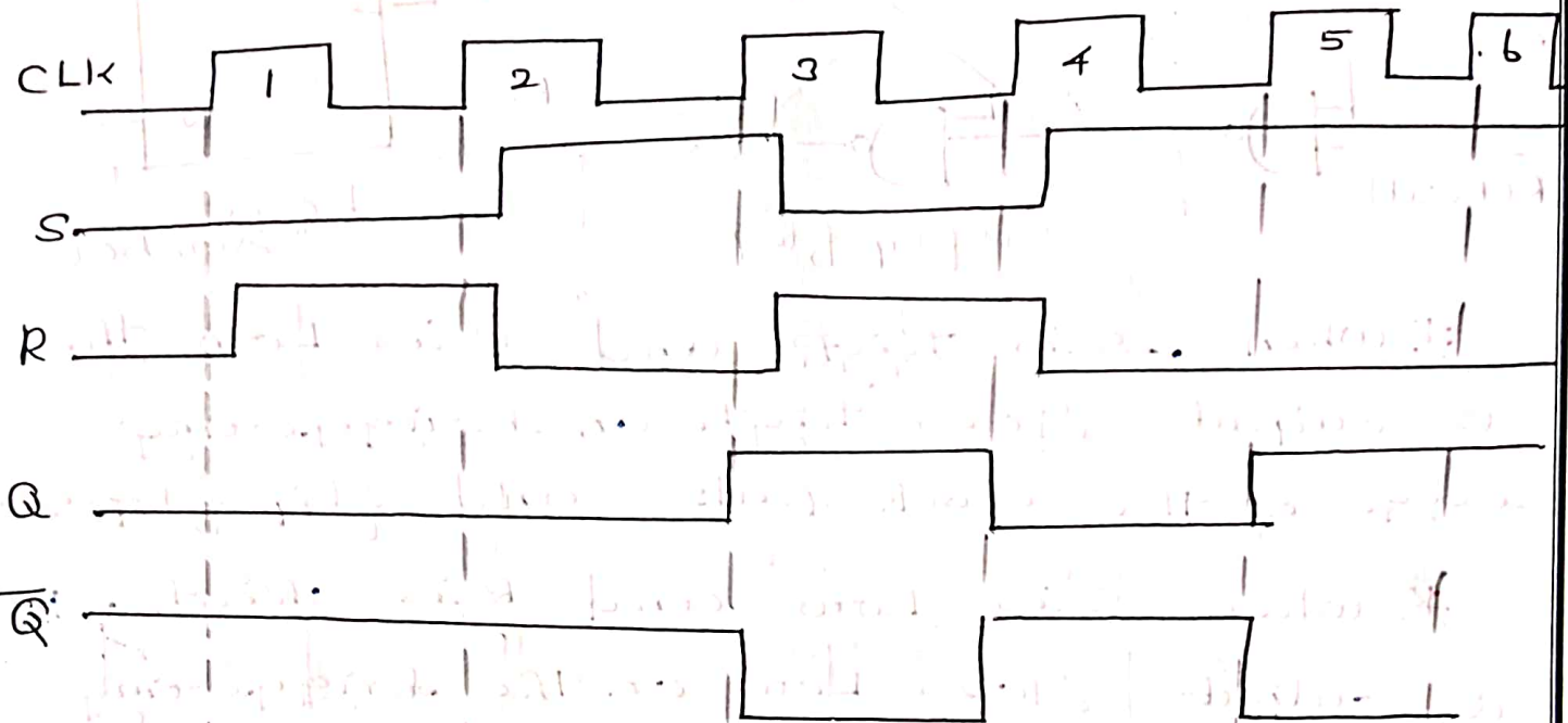
Input output wave form of SR flip flop
